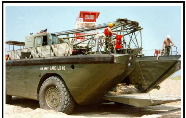
An army LARC with a crane onboard. Mars's official Military Occupational Specialty (MOS) was as a shovel crane operator, but we could imagine that the LARC was used in their amphibious projects. Each wheel of the LARC had its own diesel engine.
