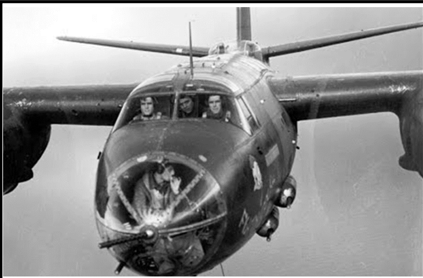
The front view of the B-26, note the bombardier under the cockpit with full view of the terrain below.
