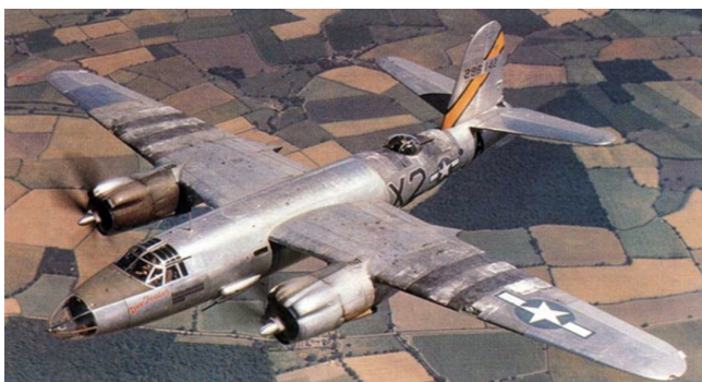
The Martin B-26 Marauder in flight. Note the glass nose for the enhanced view of the bombardier and the dorsal location of the machine gun turret for rear protection.
